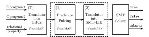
Figure 3. The Verification System: (1) the Predicate Pairing module, implementing Algorithm 1, and (2) the Translator to SMT-LIB module.
