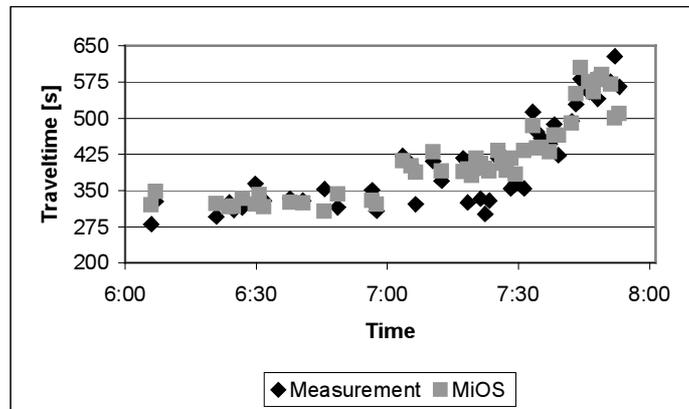
**Figure 4. Simulation result compared with travel time measurements**
