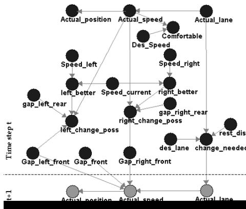
Figure 2. Structure of the BN for the Speed Decision of a driver
